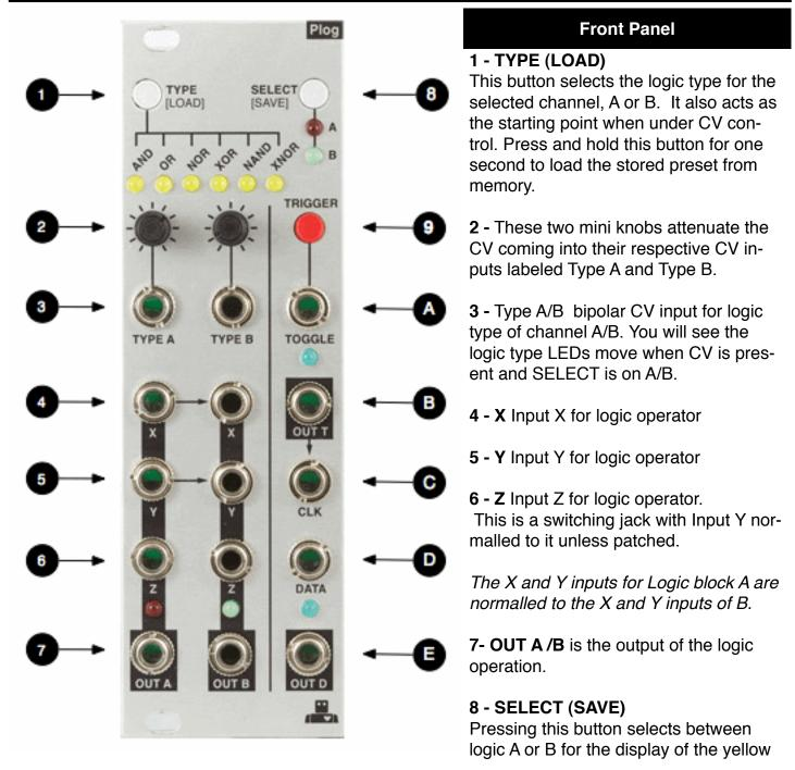
LED logic type and the operation of the TYPE button. Pressing and holding this button for more than one second will save the logic type selections into non-volatile memory.
